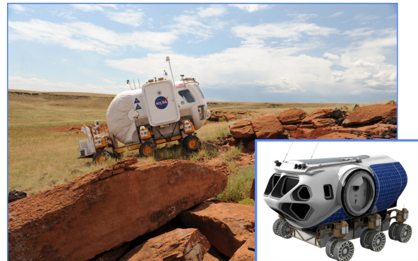
Fig. 3. A proto-type LER that has been tested extensively in simulations of 3-, 14-, and 28-day-long missions with (inset) a concept SEV.
