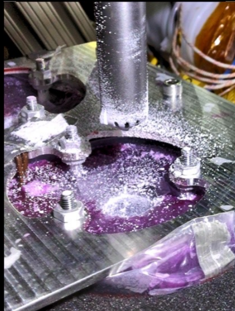
DrACO ETU (engineering test unit) end-to-end testing of drilling and sample collection in APL TPEC with water ice sample (died purple) at -180°C
