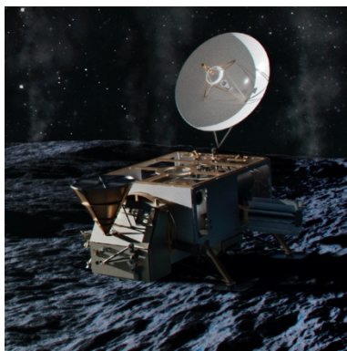
Figure 1: Artistic representation of the Orbilander concept during landed operations: HGA is deployed for sending data back to Earth and the funnel collects plume fallout.
