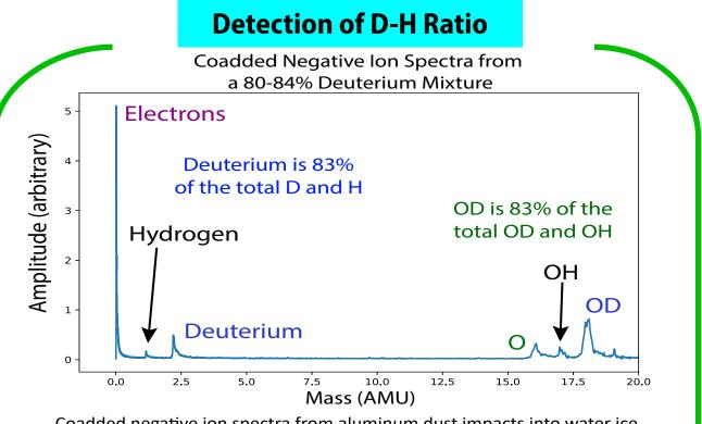
Coadded negative ion spectra from aluminum dust impacts into water ice containing 80% deuterium ions (relative to hydrogen ions). The D-H ratio is important in formation models for icy moons throughout the solar system. Our TOF was able to correctly identify the ratio of deuterium to hydrogen in a water ice sample by coadding spectra. This means that impact ionization TOF instruments on fly-by spacecraft may be able to measure the D-H ratio of icy moons and help constrain their formation models.
