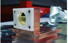
/apor deposition is used for simple ice mixtures, and ice thickness can be measured by abry-Perot interferometry.
