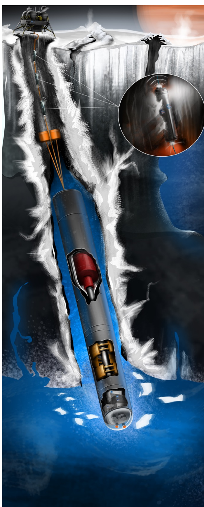
Fig. 1: Artist impression of Tunnelbot reaching the ocean, after deploying communication repeaters and the anchor [1].
