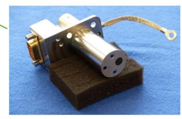
Aerothermal sensor used for ExoMars
