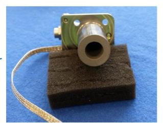
Broadband radiometer sensor used for ExoMars
