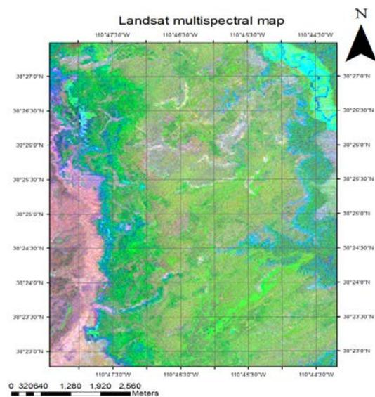
Figure 2 : Landsat multispectral data show the presence of calcite (pink color) along the inverted channels.
