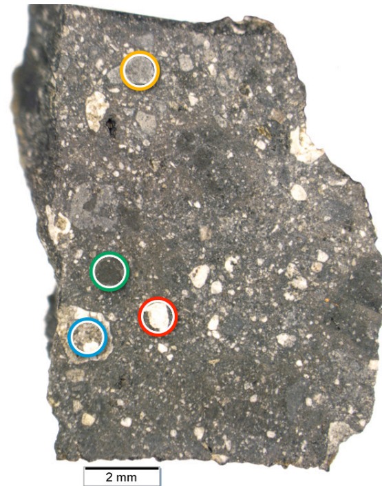
Figure 1. Optical micrograph of the NWA 7034 chip used in this study. Circled areas represent spots chosen for spectral point measurements that are shown in Figure 2.
