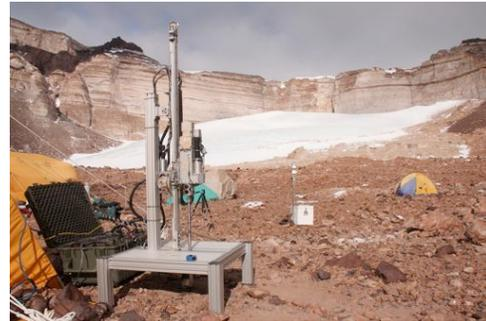
Figure 1. The Icebreaker drill, build by Honeybee Robotics being testing in University Valley in the Dry Valleys of Antarctica – a location of ice-bearing permafrost overlain by “dry permafrost”. This area is the best analog on Earth for the ice-rich regolith at the Phoenix Landing Site on Mars [1-4].
