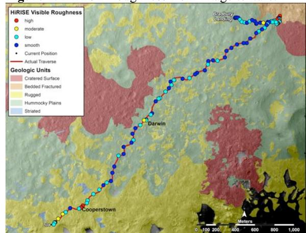
Figure 2: Terrain types near Bradbury Landing [3] and HiRISE roughness at each drive location (dots).
