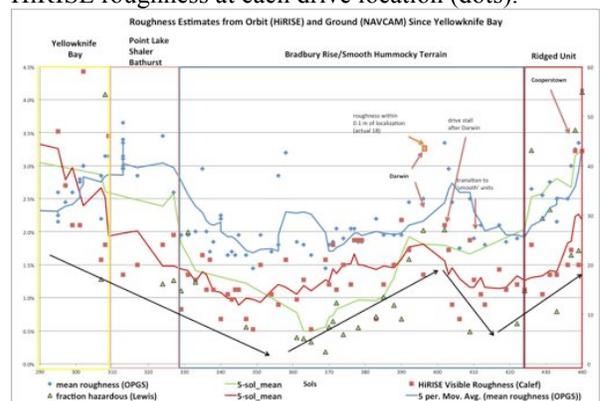
Figure 3: Comparison between orbital and ground roughness. Roughness trends between surface convexity (green triangles, K. Lewis), rover arm workspace (blue diamonds, R. Deen) and HiRISE roughness (red squares, F. Calef) appear correlative.
