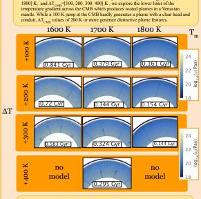
Fig. 3: The viscosity fields for the suite of reference models showing the scale of mantle plumes in 10 different temperature regimes. Notably, all models with CMB temperature jump  $\Delta T \ge 200$  K produces plumes with a distinguishable head and conduit. On average, 4.7 plumes form in each model with rise-times ranging from 10-100 Ma and total lifetimes upwards of 200 Ma.
