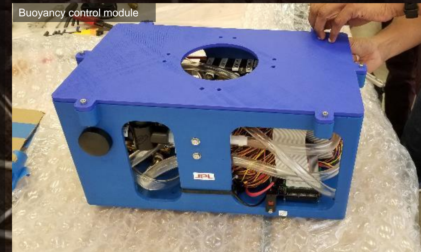
Figure 3: Buoyancy control module for adjusting balloon altitude, including pump/vent for transferring helium and logging capability of flight performance.
