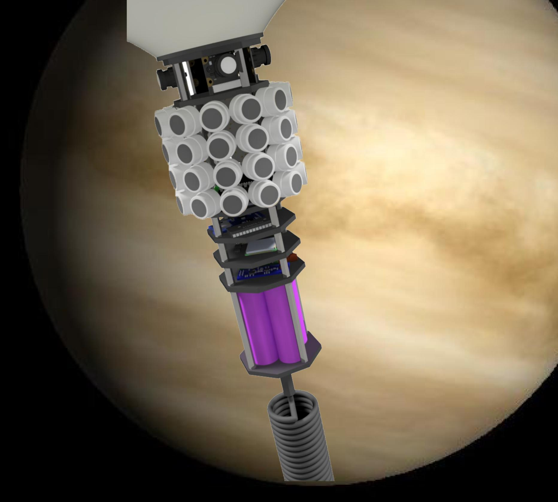
This concept is based on the design, manufacture, and implementation of a group of miniaturized independent sensing systems, with a maximum volume of one liter and a weight of around 1kg, intended for the detection of
