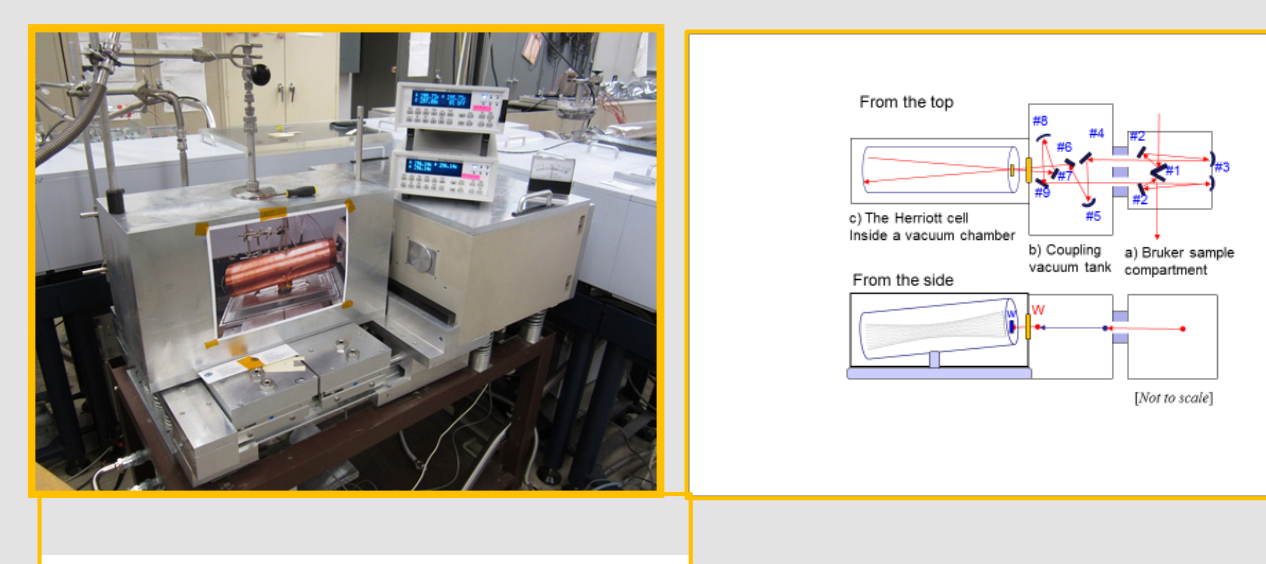
Fig. 2b. 20.9-m Herriott cell enclosed in its vacuum box and coupled to the Bruker FTS through transfer optics
