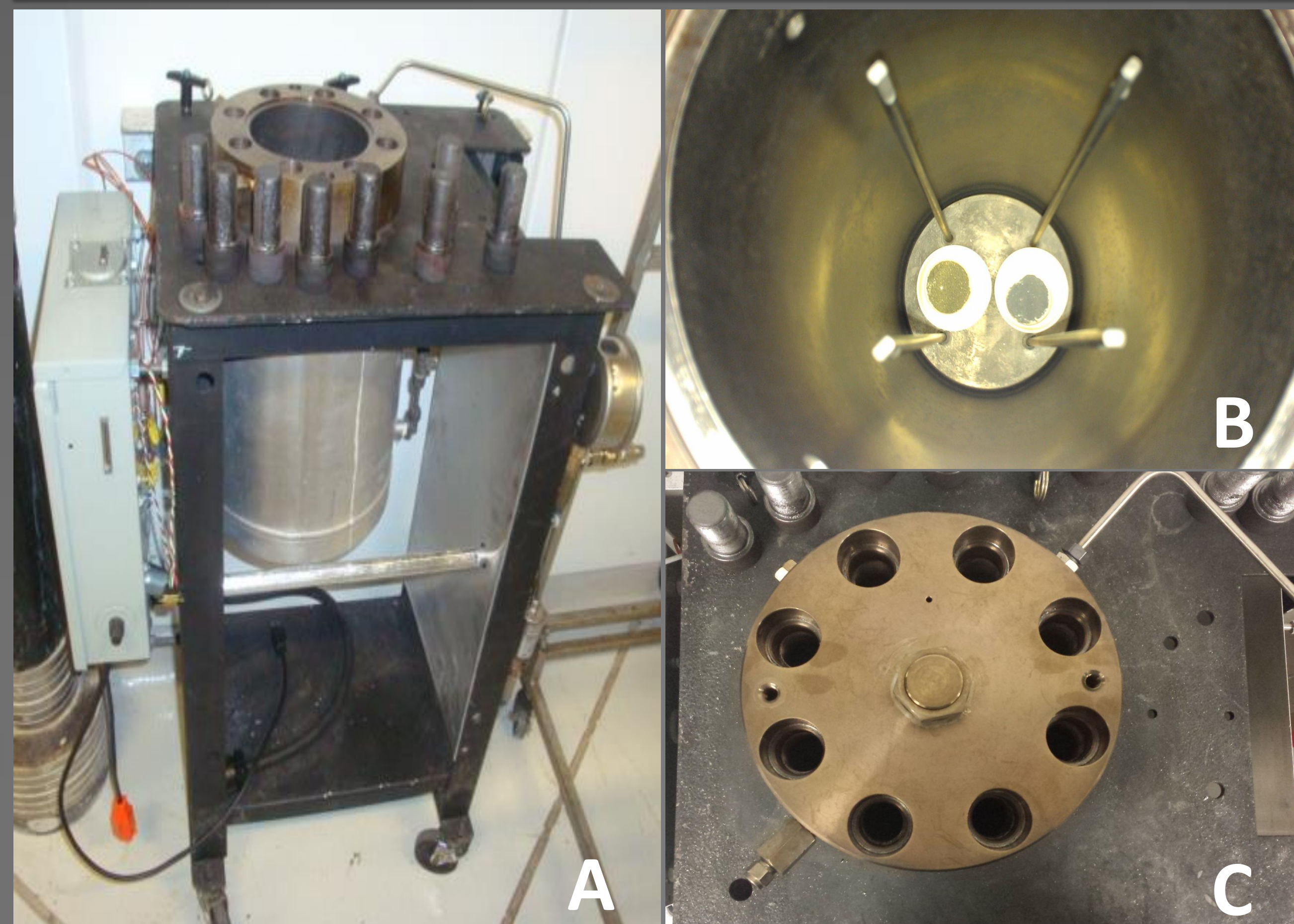
Figure 3. Images taken of the chamber where (A) shows the entire chamber and apparatus, (B) shows the interior of the chamber with removable stand for holding samples or instruments, and (C) is the lid one port used for thermocouples, other lids with optional viewports and/or throughputs can be used.
