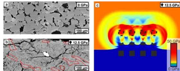
Fig. 1. SEM-BSE images of (a) unshocked and (b) shocked (12.5 GPa) Seeberger sandstone (L3). Note the total closure of pore space, the intense fracturing, and the heterogeneous distribution of diaplectic quartz glass and/or SiO<sub>2</sub> melt (red-framed areas). (c) Shock pressure distribution during pore collapse (snapshot). Note the total closure of pores (black) and the pressure amplification up to 4 times (dark red) at locations of primary pores.
