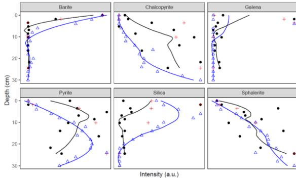
**Figure 1.** In general, mineralogical gradients deduced from MCR of LIBS spectra agree with that from gold-standard techniques. Individual data points and moving average trend lines are plotted against depth into the chimney (0 = exterior): black dots (MCR results); blue triangles (based off SEM data from a different Roane sample [6]); red crosses (XRD). (Rodriguez et al. 2021, in prep. [9])
