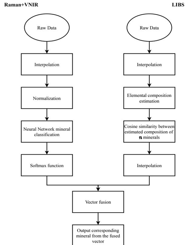
Figure 2: Simplified flow diagram showing our method for recognizing minerals from combined Raman/VNIR and LIBS spectra.
