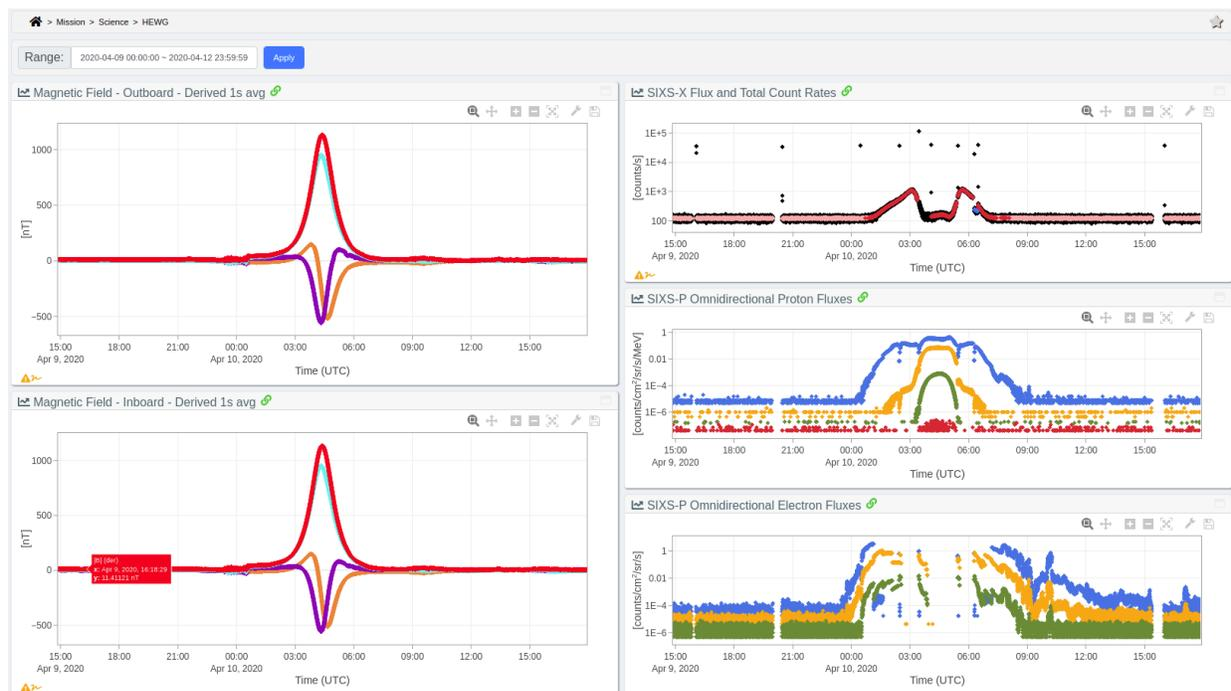
Figure 1: A snapshot of a QLA dashboard showing interactive plots of data acquired during the BepiColombo Earth flyby. All data are read “on the fly” from PDS4 products.
