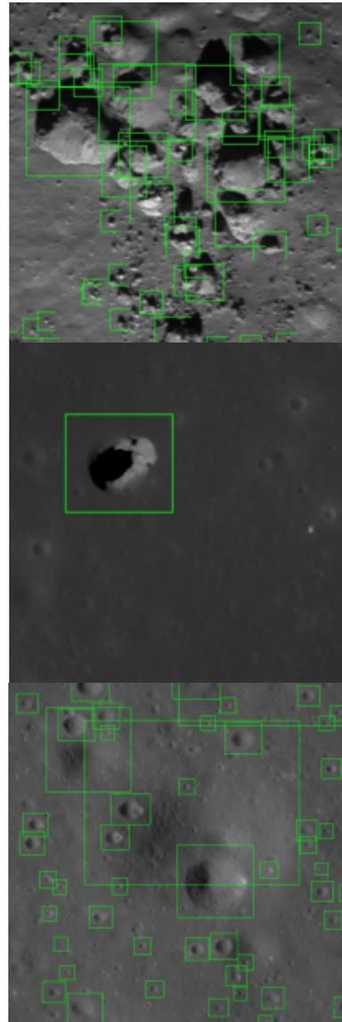
Figure 1: Sampled feature detection outputs from top to bottom, rocks, lunar pits, and craters.
