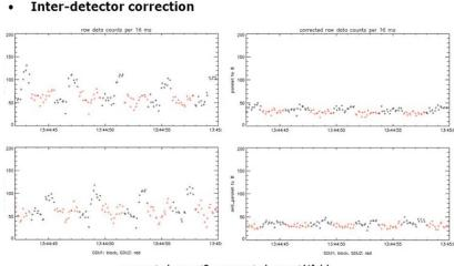
corrected\_count2 = corrected\_count1\*f\_id f\_id = D1/D2, where D1 and D2 are averages of look direction corrected raw data counts
