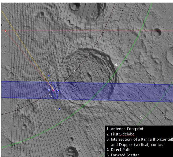
Fig. 1. Radar planning plot showing the phenomena discussed in this abstract. This demonstrates ambiguity modeled as contours, originating from the target point.
