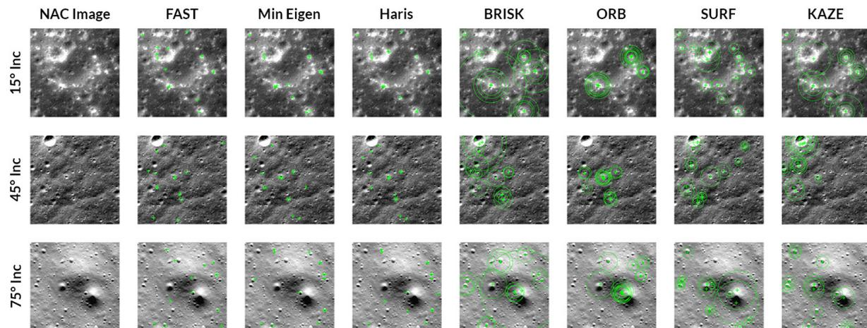
Figure 1. Application of seven feature detectors on three 256x256 pixel sub-images of LROC NAC observations with incidence angles of 15° (M109753063L), 45° (M139396321R), and 75° (M1285183949L).
