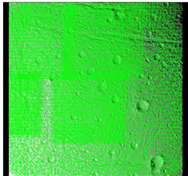
*Figure 1: Example of the dense grid of tie points (green dots) utilized in our photogrammetric solution. Tie point density varies with image density. Area shown is 135 km wide by 100 km high.*
