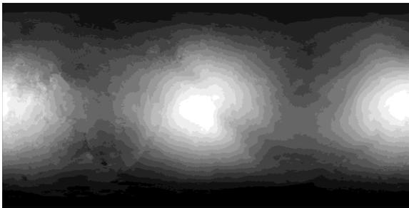
Figure 2: Preliminary global shape model from ISIS' cnet2dem. The triaxial shape is evident (degree-2 pattern). Cylindrical projection,  $\pm 90^\circ$  latitude,  $0^\circ$ - $360^\circ$  longitude. Bright regions are "higher."
