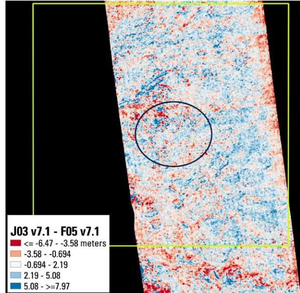
**Figure 1.** Vertical difference raster between two CTX DTMs. They are offset from one another by ~0.99 meters. This comparison is typical of elevation differences between the CTX LVS DTM and the HRSC DTM.
