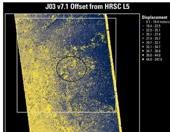
**Figure 2.** IMCORR run output illustrating the magnitude of displacement of a CTX orthoimage from the HRSC L5 orthoimage. The CTX orthoimage is displaced by a median magnitude of 29.7 meters preferentially oriented to the southeast. This comparison is typical of horizontal registration differences between the CTX LVS orthomosaic and the HRSC L5 orthomosaic.
