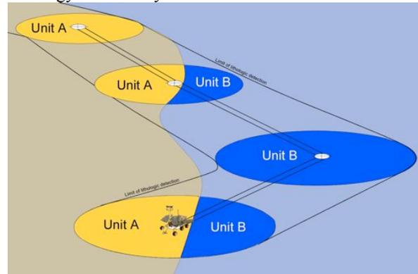
**Figure 1.** Field geologic mapping on Mars is comparable to mapping in an area of extensive cover: lithology, structure, and contacts are compared between stations and continuity derived from correlation of petrography. Elemental correlations are frequently confusing or distracting.
