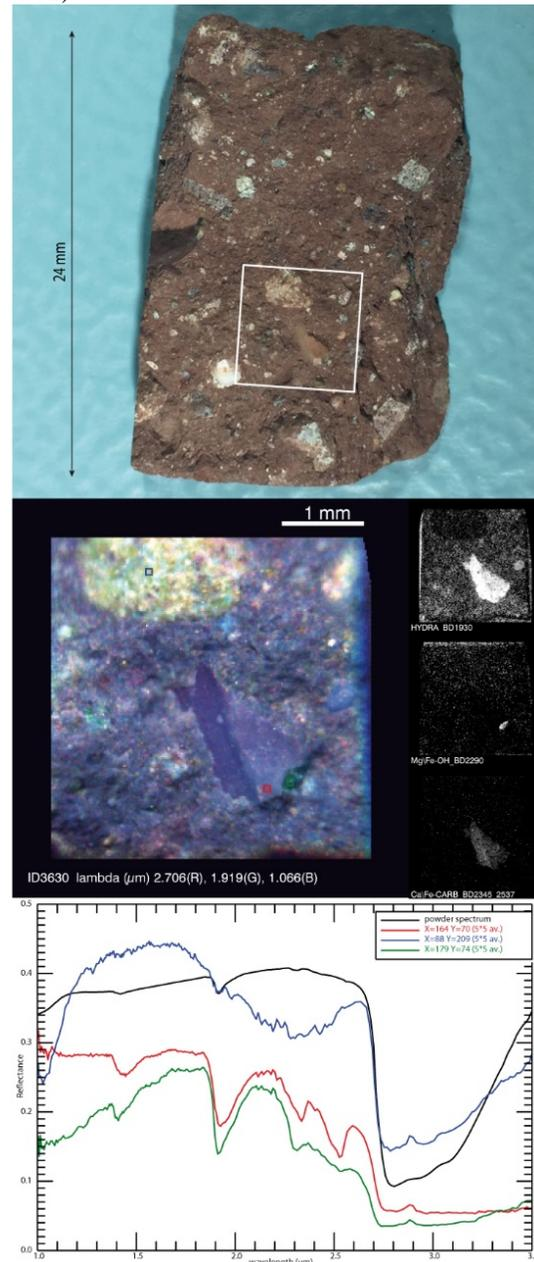
Figure 2. Example of sample characterization using MicrOmega/PTAL facilities. Top: picture of the rock surface; middle: IR composite image from MicrOmega and maps of different hydrated mineral spectral features; bottom: spectra taken from the colored squares above, and spectrum of the rock powder from the same sample.
