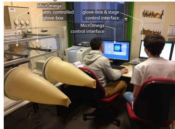
Figure 1. A view of the PTAL/MicrOmega bench during use.
