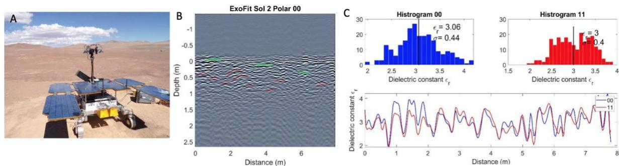
**Figure 1:** **A)** Charlie Rover (a replica of the ExoMars Rover) in the Atacama desert (Chile) during the ExoFit 2019 simulation operation campaign (Feb.-March 2019). The antennas of WISDOM are yellow in the first plan. **B)** Radargram showing the data acquired during Sol 2 of the ExoFit 2019 campaign in polarization 00. **C)** Permittivity values estimated from the surface echo amplitude along the Sol 2 traverse both in polarizations 00 and 11.
