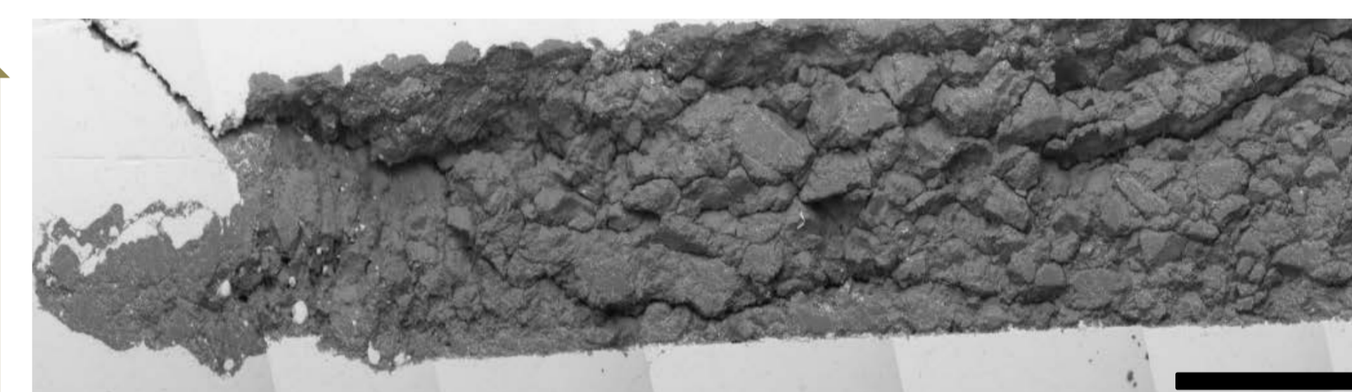
(Top) SEM-front view of opened ARMCO Fe cylinder. Dark material is olivine (Ol), cylinder material is bright. Scale bar is 500 \mu\text{m} . Dark grey arrow (left side) signifies the direction of the shock wave.
