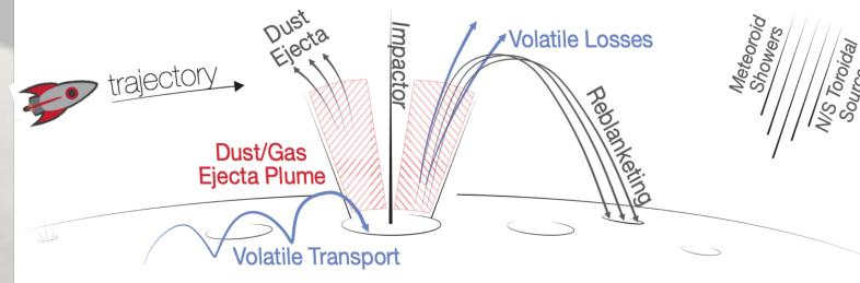
MDEX for compositional mapping of Mercury's surface: The dust particles comprising the ejecta cloud are small samples from the surface and could be used to map the chemical composition of Mercury from orbit, using MDEX, an updated LDEX instrument, a dust impact ionization timeof-flight spectrometer.
