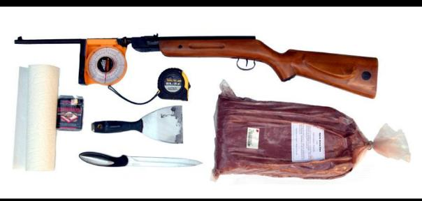
Pellet rifle with inclination meter, tape measurer. 10 kg of clay, spatulas, sharp knife for sectioning.
