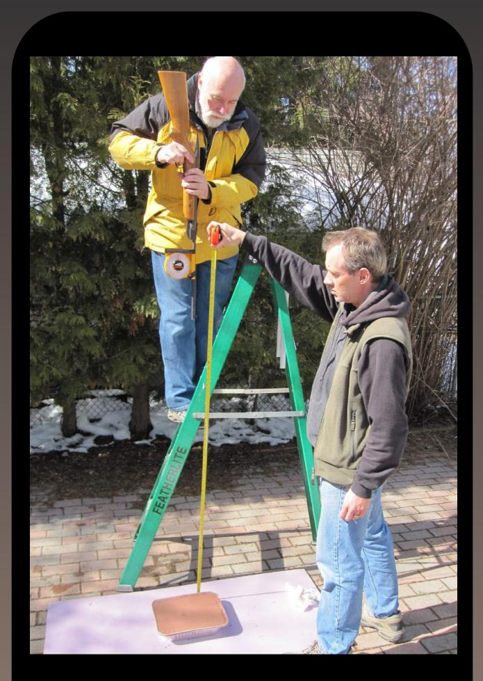
Two people, a pellet gun, inclination meter, tape measurer, and a tray of soft clay are all that is required to demonstrate cratering.
