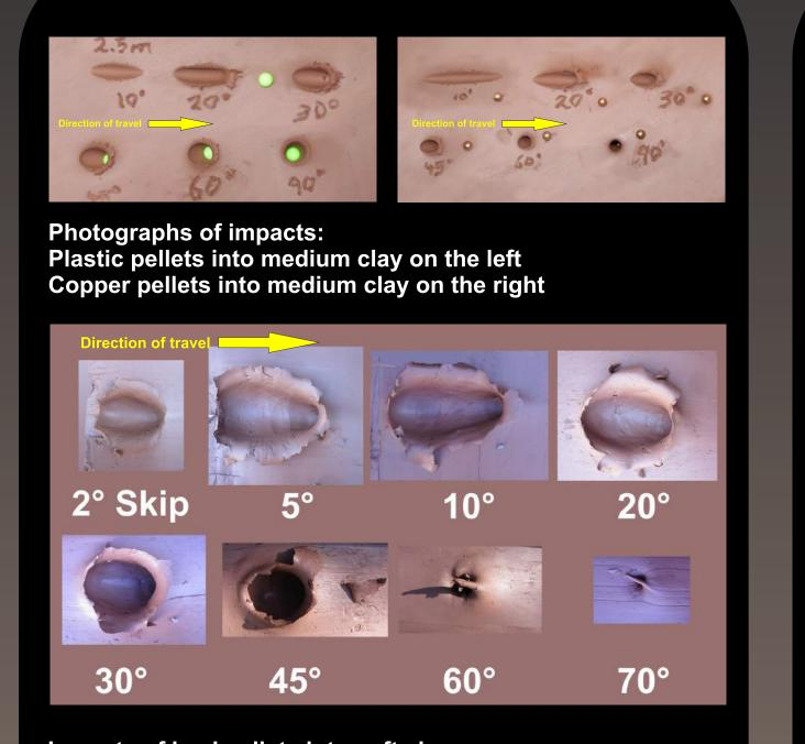
Impacts of lead pellets into soft clay.
