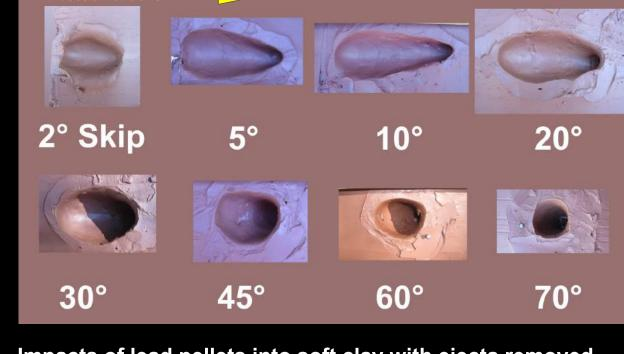
Impacts of lead pellets into soft clay with ejecta removed.
