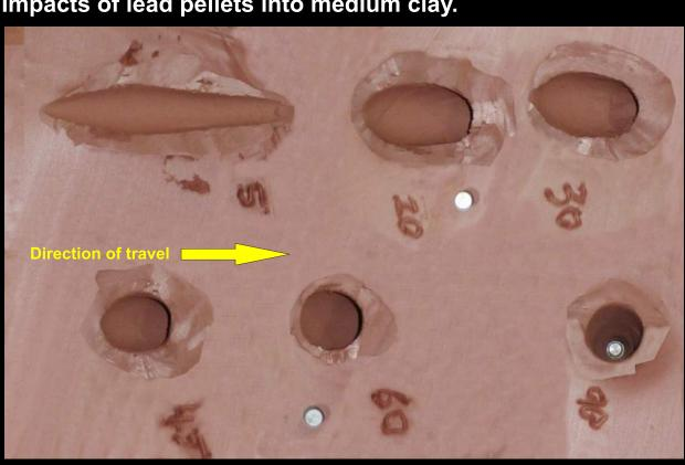
Impacts of lead pellets into medium clay with ejecta removed.
