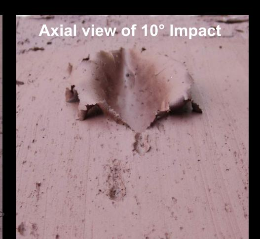
This 10° single shot of a sugar pellet (carved out of a sugar cube) shows many features that would be difficult to show with a hyper velocity gun. The main pellet produced a simple skip crater, while the tiny grains that separated in the process of being fired by the gun produced a wide range of craters, tumbles, and a splash.
