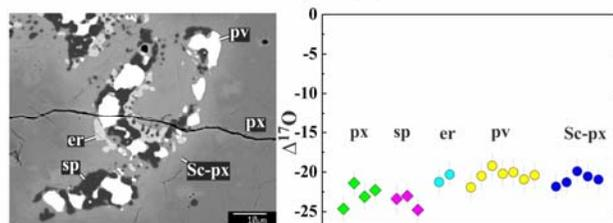
Fig. 1. (a) BSE image and (b)  $\Delta^{17}\text{O}$  values of individual minerals in the UR CAI *Al-2*. er = eringaite; pv = perovskite; px = Al,Ti-diopside; Sc-px = Sc-rich Al,Ti-diopside; sp = spinel.
