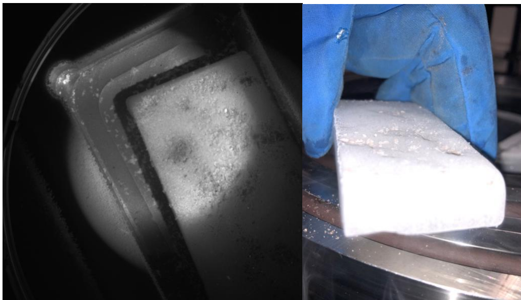
Figure 3 : (Left) Top view of the CO 2 slab during the test run. (Right) Side view of sinking areas after the experiment.
