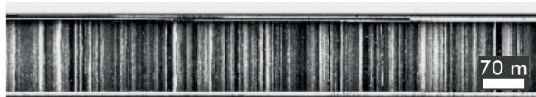
Fig 2: Scan image from a Greenlandic glacial ice core. Bright layers reveal the presence of dust, while black layers are pure ice. Image extracted from [10].
