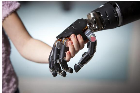
Figure 1. APL’s Modular Prosthetic Limb (MPL) is an anthropomorphic robotic end effector. See <https://www.jhuapl.edu/prosthetics>. Credit: JHU/APL.
