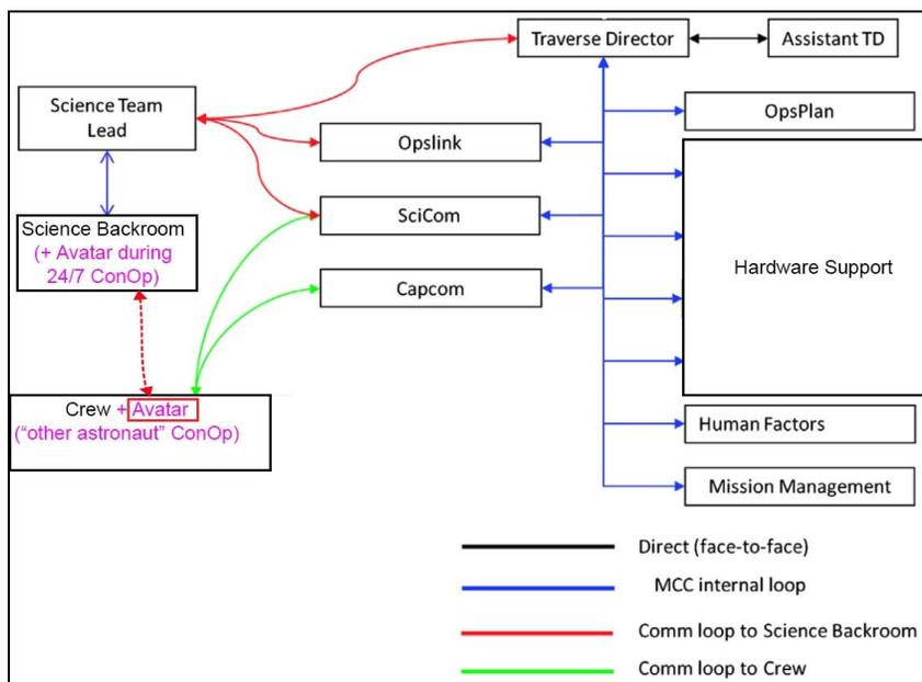
Figure 2. Basic Operations Team Organization and Communications Flow, modified from Bell et al. (2013); Avatar additions in magenta for the two different ConOps (“other astronaut” (OA) and “24/7” ConOps). The dashed red arrow indicates that the Avatar operator could have the option of conferring directly with the backroom, though this would benefit from Earth analog tests.
