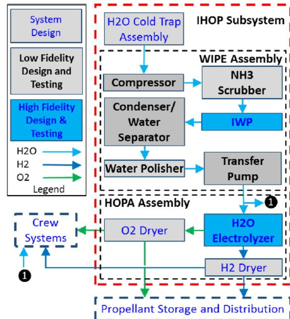
Figure 1. The IHOP concept with Water, ISRU-derived, Purification Equipment (WIPE) and Hydrogen Oxygen Production Assembly (HOPA).
