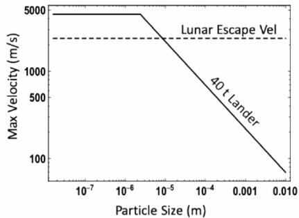
**Fig. 2:** Modeled maximum blast zone particle velocities as a function of particle size for a 40 ton lander.
