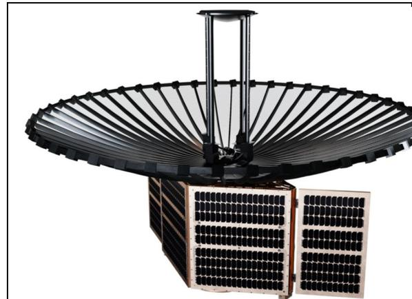
*Figure 1: Bus with wrapped rib reflector.*
