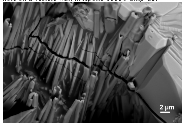
Fig. 2. Apatite needles inside the hole from Fig. 1 are embedded in Si-rich glass.
