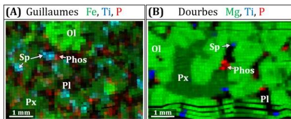
Figure 1: Red-Green-Blue (RGB) element maps for abraded patches Guillaumes (A), and Dourbes (B). Ol = Olivine, Phos = Phosphate, Pl = Plagioclase, Px = Pyroxene, Sp = Spinel.
