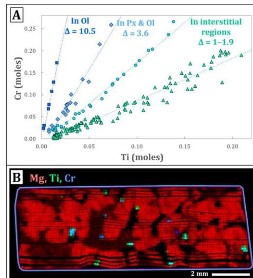
Figure 2: (A) Cr and Ti compositional trends observed for oxides in Dourbes; trend line slopes noted with  $\Delta$ . (B) RGB element map for Dourbes illustrating the spatial occurrence of Cr-rich oxides (blue - in red and dark-red mafic minerals) and Ti-rich oxides (turquoise to green - in black mesostasis regions).
