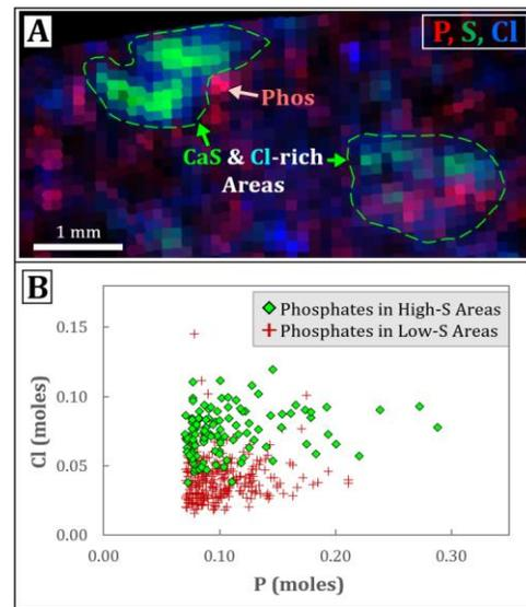
**Figure 4:** (A) RGB map for Bellegarde showing phosphates in proximity to secondary high-S regions. (B) Cl and P abundances for phosphates in Bellegarde illustrating higher-Cl phosphates are observed in proximity to secondary high-S regions (points with  $P_2O_5 > 5$  wt.%, and  $SO_3 > 2$  wt.%).
