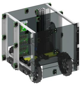
**Design:** The rover consists of four wheels, a Raspberry Pi single-board computer, control circuitry, and a chassis that holds the magnetometers in a rectangular array. In the prototype of the rover, commercial small-scale microelectromechanical systems (MEMS) magnetometers are used for magnetic field measurements. These sensors are arranged in grid to simplify the data analysis for removing the rover's own sources of magnetic interference.
