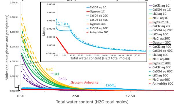
**Figure 2.** Resultant aqueous and precipitated phases (y-axis) plotted v/s total  $\text{H}_2\text{O}$  in the solution (x-axis shown in log scale). Inset shows  $\text{CaSO}_4$ , gypsum, and anhydrite on a linear scale for x-axis.
