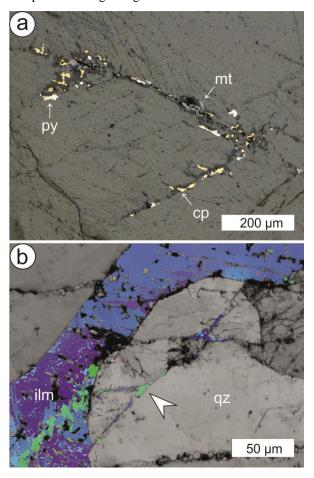
Fig. 1. Meteorite impact shock effects in iron-bearing minerals in the drill core samples. a) Magnetite (mt), pyrite (py), and chalcopyrite (cp) along planar fractures in quartz. Photomicrograph taken with reflected light of sample V2 4.2 (33 cm depth). b) Electron back scatter diffraction map displaying the crystallographic orientations of an ilmenite host grain (ilm) and ilmenite along planar fractures in quartz (qz), indicated by the white arrow. Sample V3 2.1 (5 cm depth).
