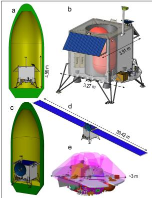
Figure 1: Views of geochronology landers for the Moon, Vesta, and Mars. a) Lunar lander in Falcon 9 Heavy 5m fairing; b) lunar lander structure accommodating the instrument deck; c) Vesta hopper with stowed solar arrays (lander and fairing dimensions are similar to the lunar lander); d) Vesta lander with unfurled solar arrays; and e) Instrument deck for a Phoenix-like lander in a 3m heat shield (pink envelope).
