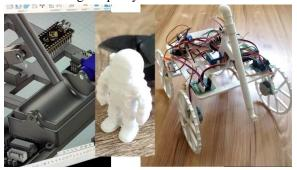
They also used Arduino sets. 28BYJ-48 Stepper Motor with ULN2003 Driver. They used Autodesk Fusion 360 to make their plans for 3D printing and for the whole design. They also printed the Spaceship of Watney.
