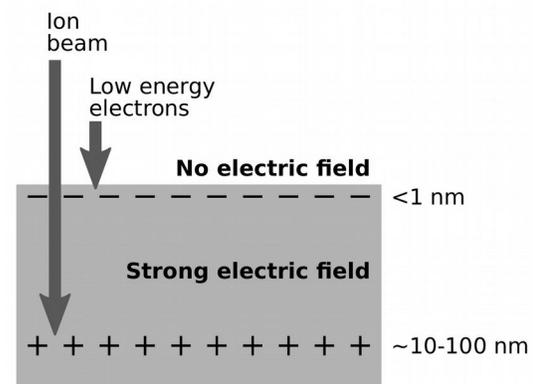
Fig. 1. Cartoon showing how an electron gun can neutralize a target irradiated by an ion beam, yet still create an internal electric field that could cause dielectric breakdown (from [11]).
