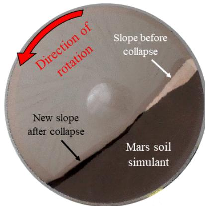
**Fig. 1** Apparatus used in slope stability experiment. This figure is a composite of the frames just before and just after slope failure to illustrate the changing slope. Sand from the white shaded area avalanches and is deposited downslope in black shaded area. The static angle of repose is measured in the frame just before collapse and the dynamic angle of repose is measured in the frame following the avalanching of sediment.
