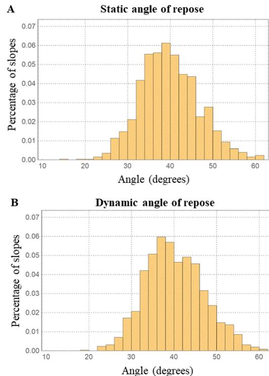
**Fig. 2** Histogram showing the distribution of angles of repose measured in dry Martian sediment simulat (i.e. zero adsorbed water). A) The static angle of repose, or the maximum steepness where a slope remains stable, is measured in the frames immediately preceding a slope failure event. B) The dynamic angle of repose, which sediment reaches after slope failure, is measured in frames directly following a slope failure event.
