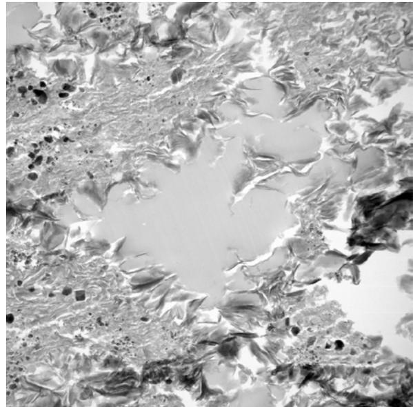
Figure 1. Bright-field STEM image of L2098B1 showing coarse-grained phyllosilicates and a large aggregate of carbon nanoglobule material. The field of view is 10  $\mu\text{m}$ . The sub- $\mu\text{m}$  dark grains are FeNi sulfides.
