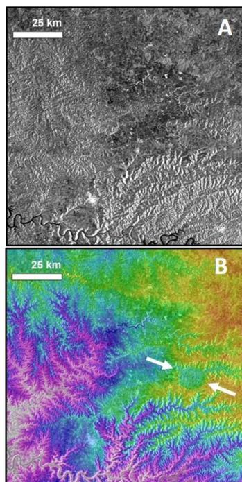
**Fig.3:** (A) Sentinel-1 radar image and (B) a 30 m resolution DEM overlaid on the radar image of the Vargeão Dome crater (Brazil). Arrows highlight the position of the crater.
