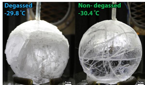
Fig. 2. Final crack coverage comparison for degassed and non-degassed water spheres frozen at -30°C.
